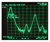
**Figure 5a:** 1 kHz ripple in span to 1300 Hz
