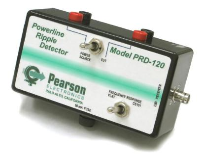
**Description.** The Pearson PRD-120 facilitates the measurement of power line ac ripple using a frequency selective voltmeter, i.e., EMI receiver or spectrum analyzer. In so doing, it greatly simplifies both the manual and automated measurement of injected ripple in such standards as MIL-STD-461 CS01/CS101, RTCA/DO-160 section 18 and MIL-HDBK-704-2 through -6.
