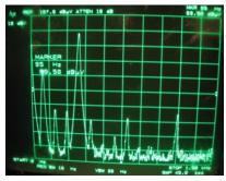
**Figure 4a:** View of 6.3 Vrms 100 Hz ripple on a 400 Hz 115 Vrms bus, using the PRD-120
